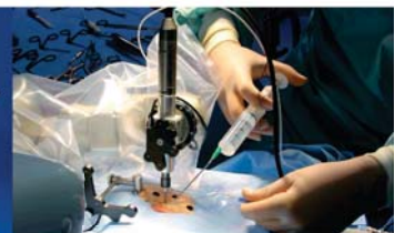
Novel surgical platform for minimally invasive interventions in the ear
